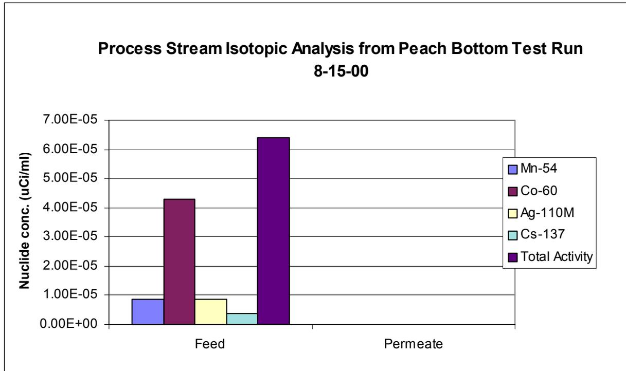
Fig. 3: Activity removal from L-mode test run at Peach Bottom
