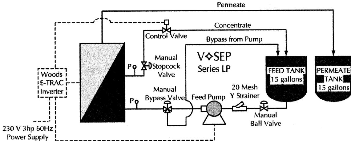
Fig. 2 Concentration Mode System Configuration
