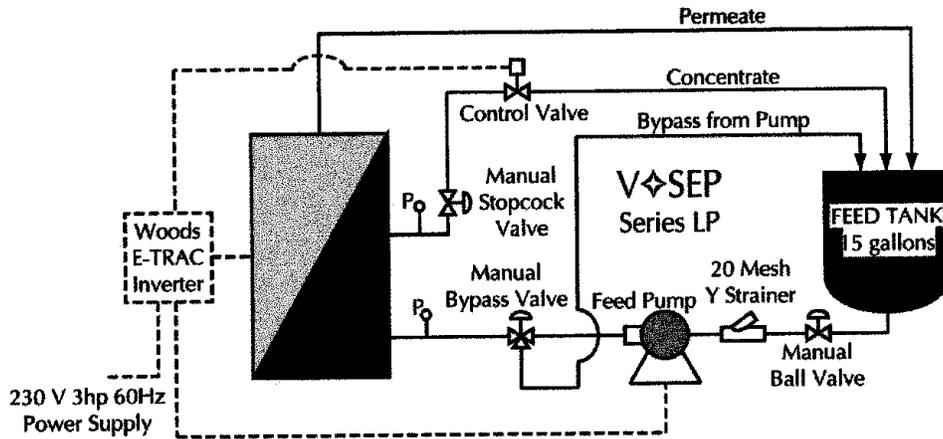
Fig. 1 “Line Out Study” System Configuration
