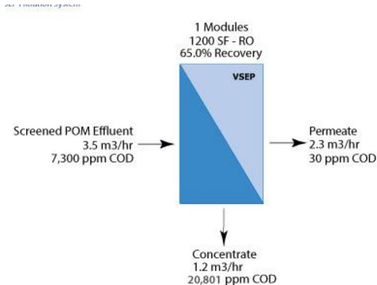
The reject from both stages of RO is sent back to compost piles where the concentrated nutrients are further absorbed into the fiber media. VSEP is producing approximately 75% of the volume as clean water and is leaving a reject volume of about 25%. The clean water is used as boiler feed water to make steam, or for irrigation.
