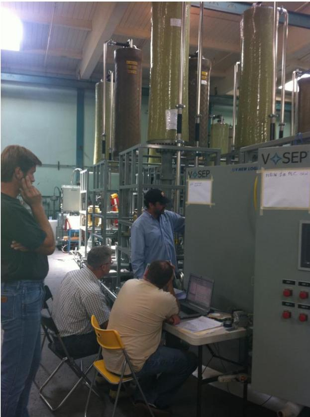
VSEP is a cross flow membrane that is able to produce economical flow rates and reliability with fouling resistance due to the vibrations. The membrane vibrates at a 3/4" displacement at 50Hz. The vibration keeps the turbulent flow at the surface of the membrane allowing large molecules to continue movement away from the surface, avoiding fouling and allowing clean water to pass through the membrane.
