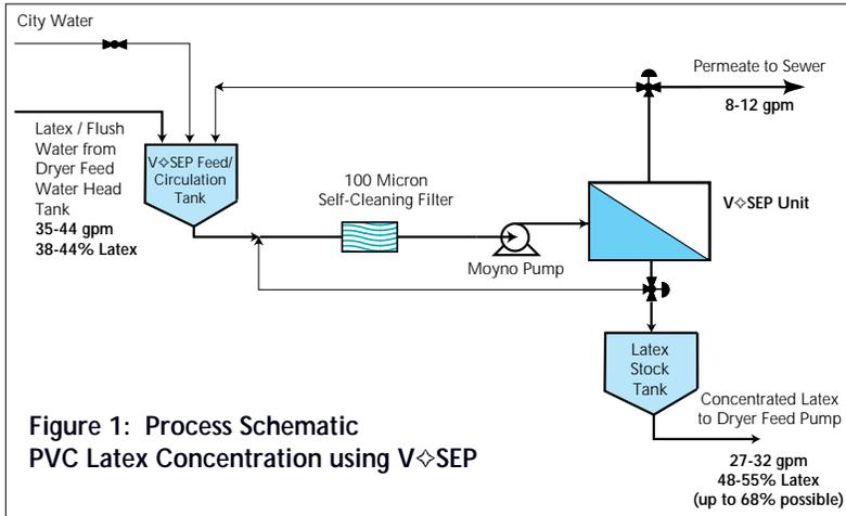
**Figure 1: Process Schematic
