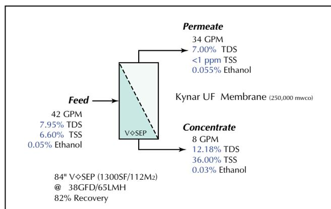
**Typical performance of a single V diamond SEP modular Series i membrane filtration system**
