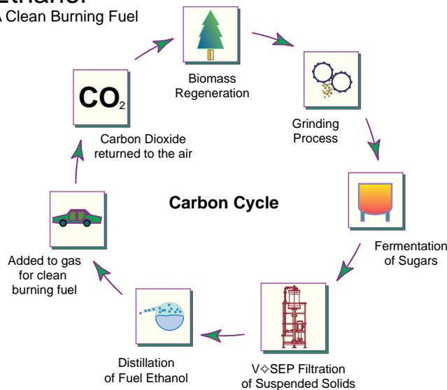
Removal of the solids from the aqueous stream can take place before or after distillation. Removal prior to distillation has the benefit of keeping the distillation equipment clean and free of solid residue build up. The aqueous stream can then be treated with simple evaporation technology.
