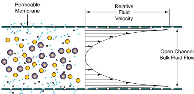
**The relative performance of V◇SEP modular Series i membrane filtration compared to crossflow**
