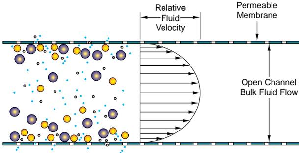
Tangential Flow Pattern in Vibratory V◇SEP Membrane Systems
