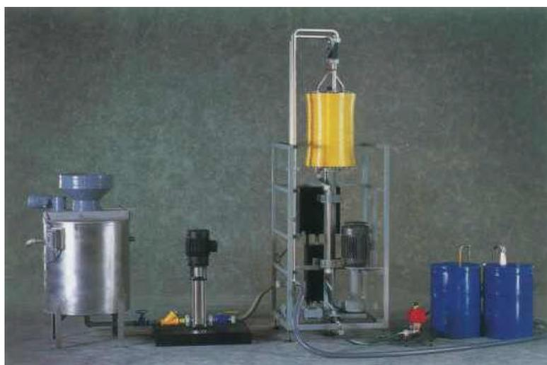
Figure 5: Typical VSEP Setup
