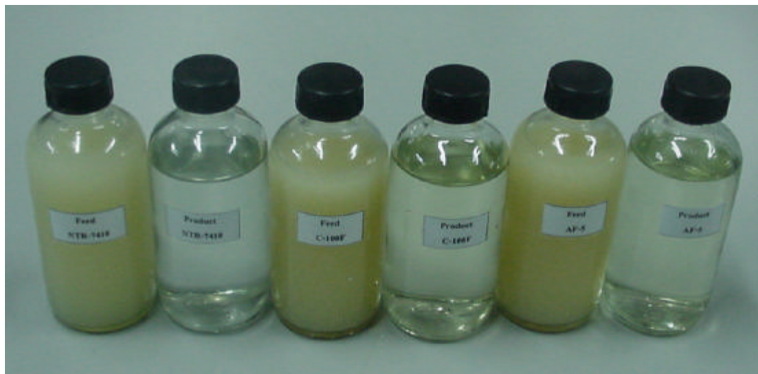
Figure 7 Feed and Product of each membrane (NTR-7410, C-100F and AF-5)
