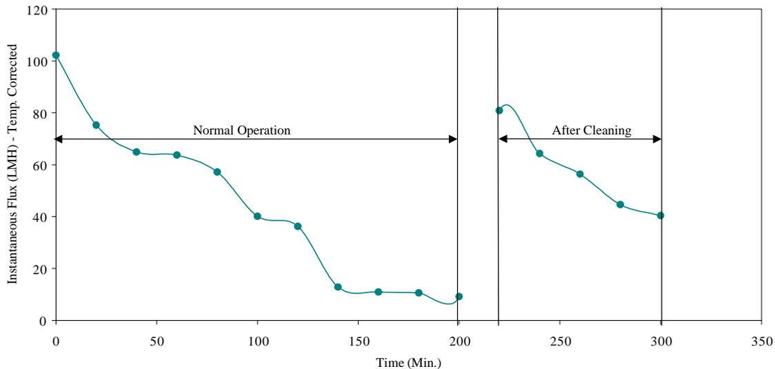
Figure 8 Flux and cleaning Performance for NTR-7450 membrane
