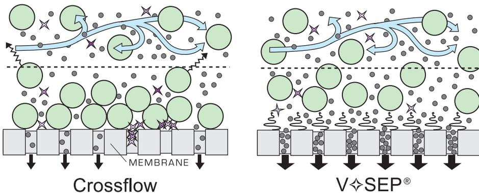
**VSEP overcomes fouling problems commonly associated with membrane filtration by using vibration to create high shear at the membrane surface.**
