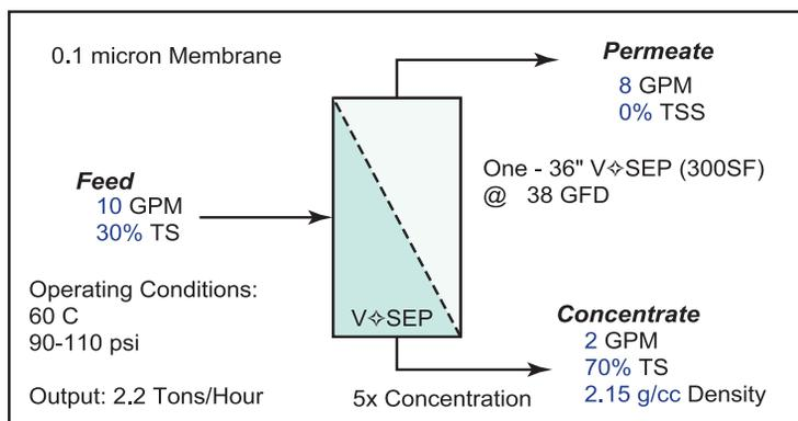
A typical Titanium Dioxide Flow Diagram.
