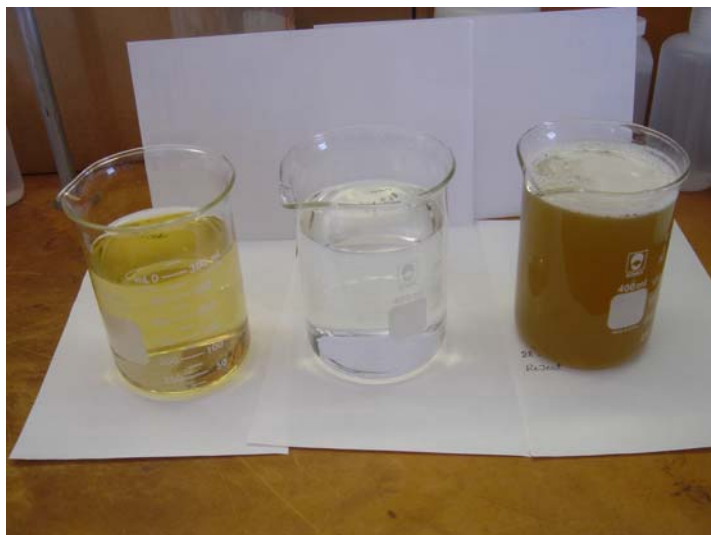
FIGURE 5 Comparison of RO Reject (VSEP Feed), VSEP Permeate and VSEP Reject from the Pilot VSEP Unit (85% Water Recovery)
