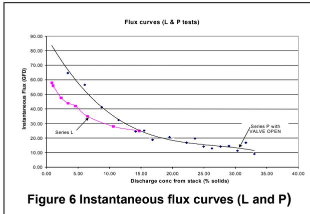
The P flux curve was slightly higher than the L curve at low concentrations but lower at high concentrations. Flux declined from around 70 GFD (120.7 l/m<sup>2</sup>/h) at the feed concentration to around 10 GFD (17.2 l/m<sup>2</sup>/h) at 33% solids (Figure 6).
