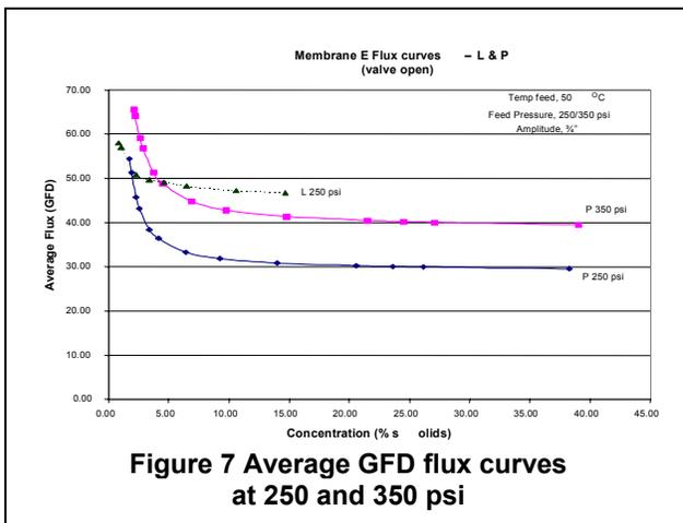
The average flux to concentrate from 1.4% to 39% was around 30 GFD at 250 psi (51.7 l/m<sup>2</sup>/h, 1700 kPa) and around 40 GFD at 350 psi (68.9 l/m<sup>2</sup>/h, 2410 kPa) (Figure 7). This concentration relates to a recovery of over 96%. Both feed pressure and temperature were found to have a significant impact on flux.
