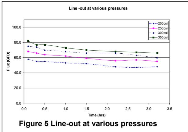
The graph in Figure 5 shows the performance of the membrane at various pressures during the “Line Out Study”. The flux rate increased steadily as the feed pressure was increased. The relative decline in flux (i.e. starting flux – ending flux) appeared to be similar at all the feed pressures tested. The pilot-plant trials were conducted with a feed pressure of 250psi (1725 kPa) – due to feed pump constraints.
