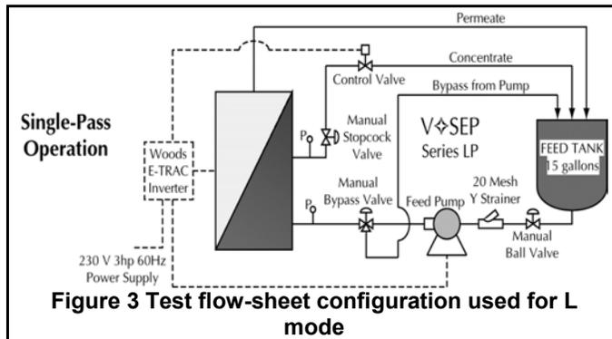
Figure 3 Test flow-sheet configuration used for L mode
