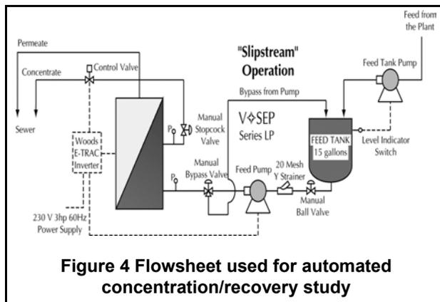
**Figure 4 Flowsheet used for automated concentration/recovery study**
