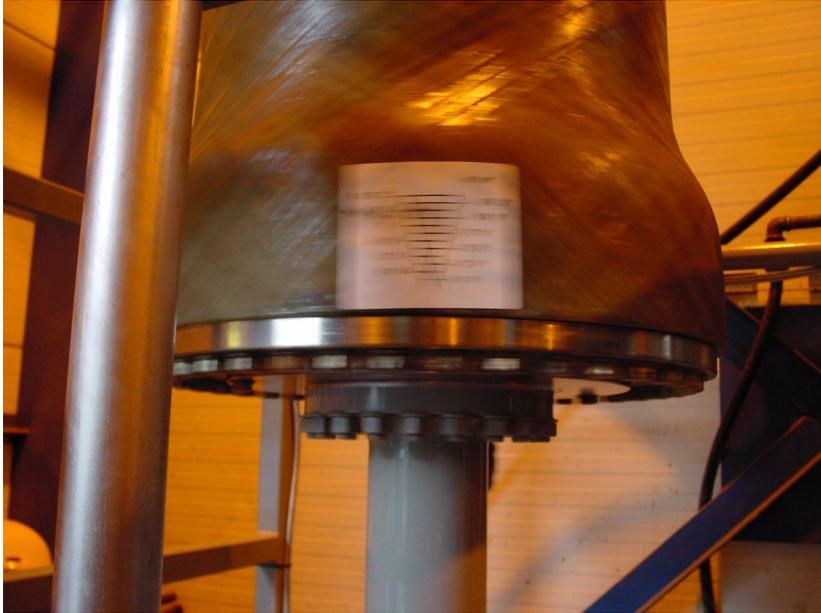
Figure 7: *Vibrating Shear Enhanced Proces (VSEP) membrane module in operation*
