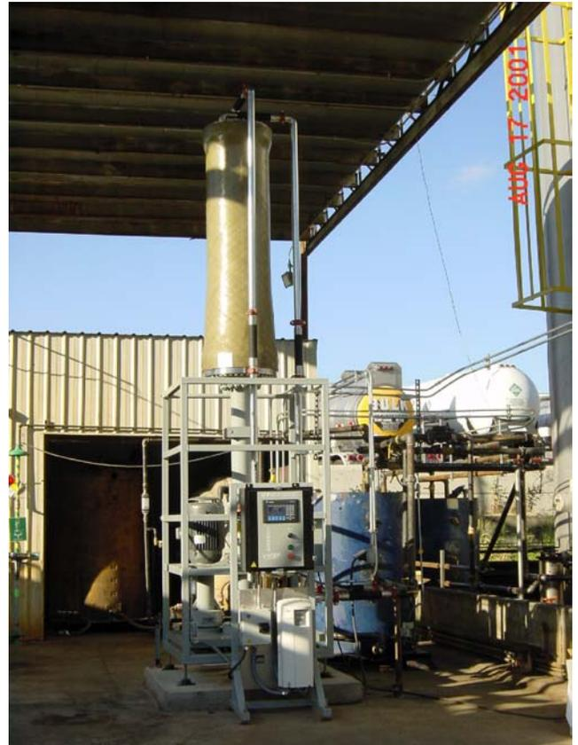
some configurable parameters be reached. The control stand contains the PLC, Operator display and terminal strips for wiring connections to instrumentation.
