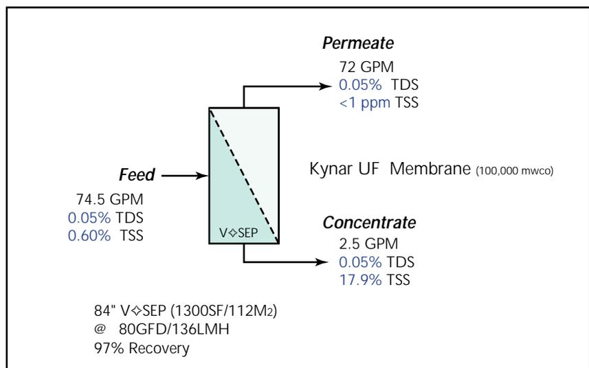
**Typical V-SEP performance on Mining and Excavation Drainage**
