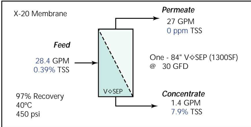
contents of the filter pack are concentrated and volume reduced until the desired % recovery is reached. Each V◇SEP unit can process about 39,000 gallons per day. The permeate can be sent back around as the initial rinse water or used for other purposes in the plant. The concentrate contains 5-15% of valuable metals that can be recovered using other techniques and then recycled.
