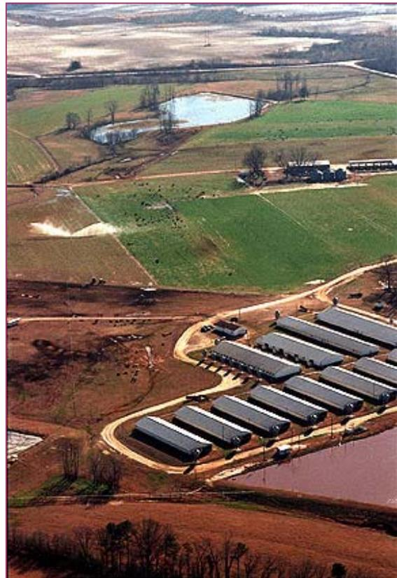
Aerated lagoons are sometimes used in conjunction with anaerobic and/or facultative lagoons to provide further polishing of effluent. Naturally aerated lagoons are less than 1.5 m deep to promote light penetration and oxygen transfer. The surface area of these ponds must be very large and they are rarely practical for treating intensive livestock effluent. Mechanical aerators can be used to promote aerobic conditions. However, this is very expensive.
