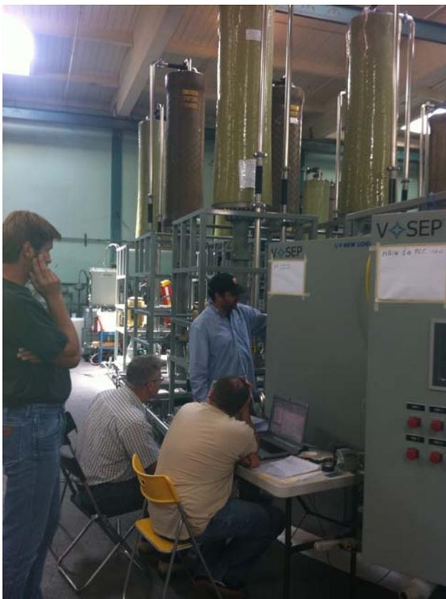
The VSEP is a cross flow membrane that is able to produce economical flow rates and reliability with fouling resistance due to the vibrations. The membrane vibrates at a 3/4" displacement at 50Hz. The vibration keeps the turbulent flow at the surface of the membrane allowing large molecules to continue movement away from the surface, avoiding fouling and allowing the water to pass through the membrane.
