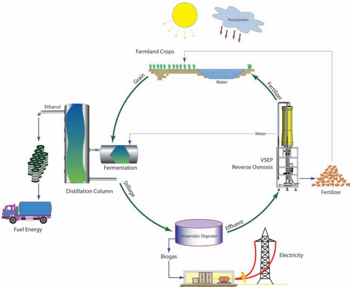
The raw materials used for the process are grains that are grown locally. Because of this transportation costs and environmental impact are low. In order to get good methane gas production in the bio-digester, they also add slaughterhouse wastewater and milk wastewater hauled from local companies nearby.
