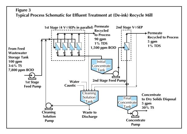
The VSEP produces a concentrated waste stream at a flow rate of 5 gpm which is discharged. The concentrated stream contains approximately 30-35% by weight of total solids (TS). The VSEP treatment system also generates a permeate stream of about 95 gpm which is recycled into the process. The feed to the VSEP unit has about 3 to 6% solids (TS). The permeate concentration of fibers is less than 1% of TS, well below the design criteria for process recycle requirements.
