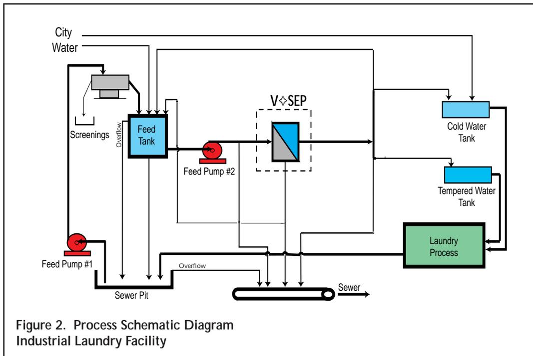
Figure 2. Process Schematic Diagram
