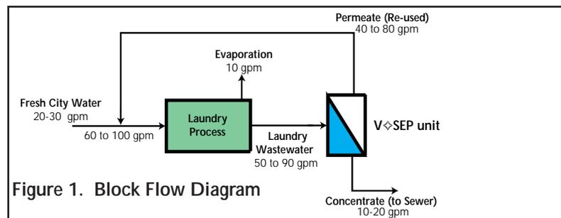
Figure 1. Block Flow Diagram
