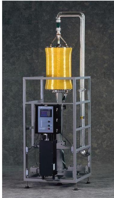
**The VSEP system takes up just 20 square feet of floor space and requires enough power to drive a 20 hp electric motor.**
