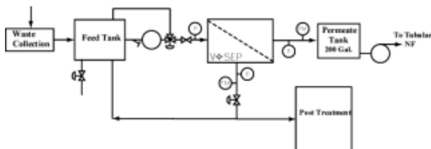
Figure 4: Simplified flow diagram of industrial unit. There is a peripheral CIP skid not shown in this diagram but was part of the purchased system.
