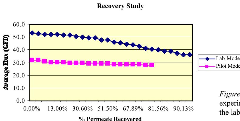
*Figure 2: A comparison of the experimental data collected on the lab and pilot VSEP units.*
