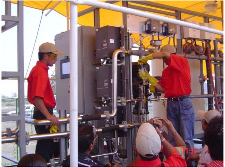
The two-stage RO process in this case reduced the Chemical Oxygen Demand (COD) in the leachate from 10,000 mg/L to only 17 mg/L in the final treated water. The total dissolved solids (TDS) in the leachate was reduced from 26,000 mg/L to about 55 mg/L.
